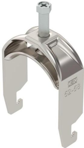
Clamp clip with U-foot, metal pressure trough with rounded edges to protect the cable. For vertical and horizontal mounting of 1 single cable on a C-profile rail. For slot width 18–22 mm. With 1-start screw thread on pressure trough, universal hexagonal screw head WAF10, with slot and cross recess. Suitable for mounting indoors and outdoors. We recommend the use of a counter-trough.
