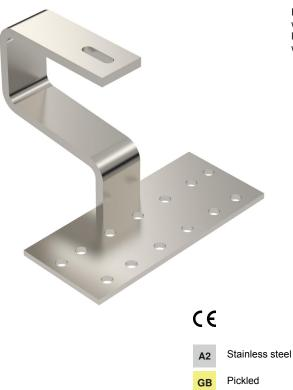
Heavy roof hook to mount photovoltaic modules on pitched roofs in combination with the TP 45 support profile. Suitable for tiled roofs. Fastening on support profile through bolt with hammer nut, type SKSHM A2. Mounting on rafters with TKS wafer-head screws.
