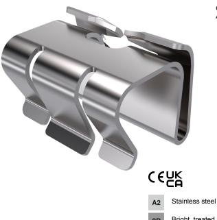
Cover clamp for secure fastening of covers on cable trays and cable ladders. At least 6 cover clamps should be mounted for each 3 metres of cover.
