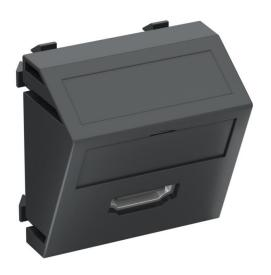
Multimedia support with one HDMI connection socket, slanting cable outlet, with labelling panel, HDMI socket with screw connection. Support plate with locking fastening, suitable for horizontal and vertical installation in the system environment
