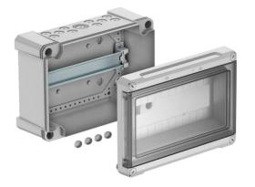
Small distributor for surface mounting, for the current sub-distribution in interior and exterior areas, according to IEC 439-3. With pre-mounted 35 mm hat profile rail. IP66 protection type and IK08 protection rating. Transparent cover to screw on, with cut-out. Including 4 screw cover caps.
