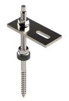
Hanger bolt set to mount photovoltaic modules on pitched roofs in combination with the TP 45 support profile. Suitable for fastening in the wooden substructure of corrugated roofs made out of plastic, tin or fibre cement. Set consists of hanger bolt with pre-mounted EPDM seal, adapter plate for the support profile and additional nuts for the optional height adjustment. Fastening of the support profile with screw with slot nut, type SKS HM (please order separately).
