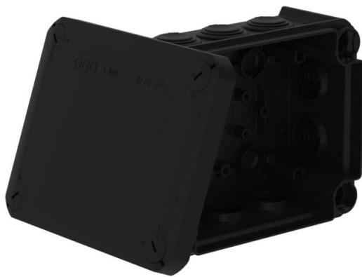
Junction box for the connection of cables and lines indoors and in protected outdoor areas. Rectangular design with plug-in seals to the sides and knock-out entries in the bottom. Suitable for wall and ceiling mounting and on mounting panels. With the option to fasten inside and to mount via the corner domes. Cover with quick lock, sealable. Made from halogen-free and UV-resistant materials.
