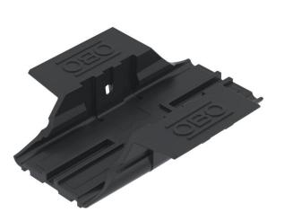
Adapter for TP 45 support profile, for mounting on UniBase universal stand. Toolless mounting through snapping. With side holes for optional screwing. Tooless mounting and dismantling of the support profile possible. With non-slip support surface.
